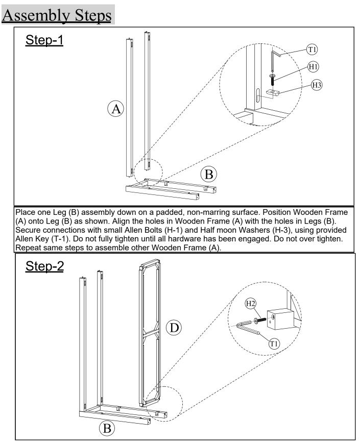
Position Bottom Shelf (D) onto Leg (B) assembly as shown. Align holes in Leg (B) with the holes in Bottom Shelf (D). Secure connection by inserting large Allen Bolts (H-2) into the bottom of the Leg (B) and engage with Bottom Shelf (D). Engage all bolts first, then loosely tighten using provided Allen Key (T-1) Do not over tighten.
