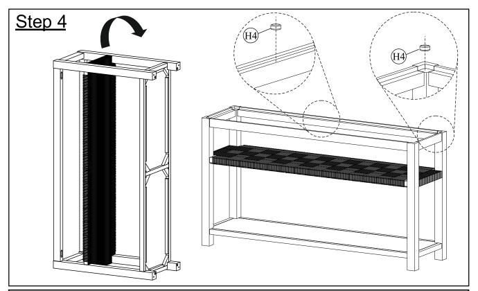
Using a second person to assist you, carefully turn the table into upright position. Add Adhesive Glass Bumper (H-4) at center & all corners on to the top frame.
